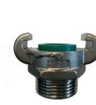
Claw distance: 42 mm Working pressure: 10 bar / 145 Psi Profiled seal DIN 3489-D: FPM Male thread EN 10226-1 / DIN 2999, BSPT (not complying with DIN 3489)
