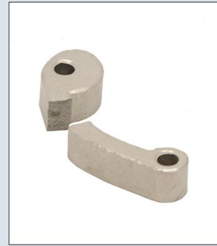
Fractured sintered handle
