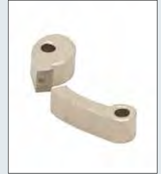
Fractured sintered handle
