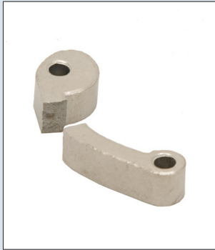
Fractured sintered handle
